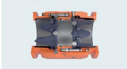
Unit in operating mode with weak-bolts intact and valves open. The two halves of the unit will part when a preset load, or a load/internal pressure combination is reached and the weak bolts break.
